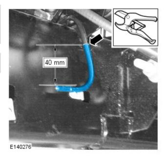
10. CAUTION: Make sure the air line insert is in the correct orientation, failure to follow this instruction may cause damage to the component.
