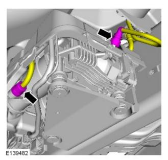
**25.** If installed, remove and discard the air line link pipe.
