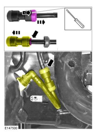
**26.** Disconnect the air line and 2 electrical connectors.
