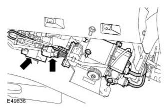
7. CAUTION: Make sure that the cover is correctly located behind the bracket as shown. Failure to follow this instruction may cause noise/vibration issues.
