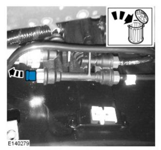
13. Install the new air line link pipe.
