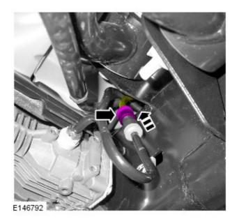
15. CAUTION: Make sure the air lines and wiring harness are not trapped between the suspension compressor mounting bracket and the chassis, failure to follow this instruction may cause damage to the vehicle.
