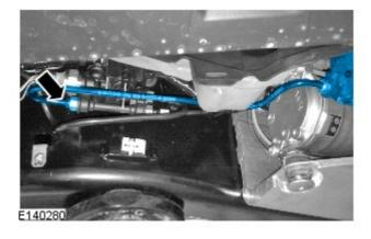
14. Connect the new air line link pipe.
