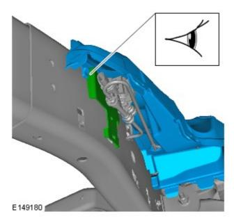
30. CAUTION: Make sure the air lines and wiring harness are not trapped between the suspension compressor mounting bracket and the chassis, failure to follow this instruction may cause damage to the vehicle.
