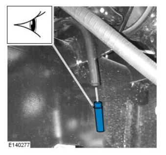
**36.** Install the new air line link pipe.
