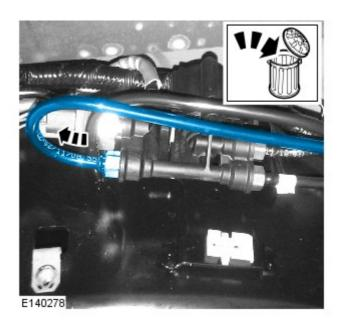
12. CAUTION: Do not remove the blanking plug until after the connector is tightened.
