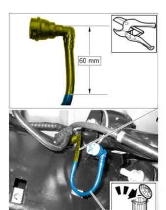
35. CAUTION: Make sure the air line insert is in the correct orientation, failure to follow this instruction may cause damage to the component.
