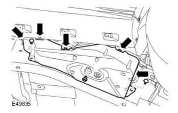
5. CAUTION: Make sure that the 3 suspension compressor mounting nuts in the chassis rail are not damaged or corroded. If required, install the nuts.
