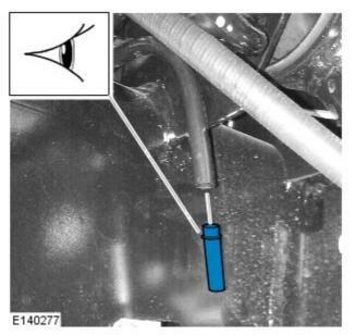
**11.** Remove and discard the air line and connector from the valve block.
