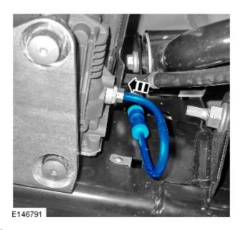
17. CAUTION: Make sure the air lines and wiring harness are not trapped between the suspension compressor mounting bracket and the chassis, failure to follow this instruction may cause damage to the vehicle.
