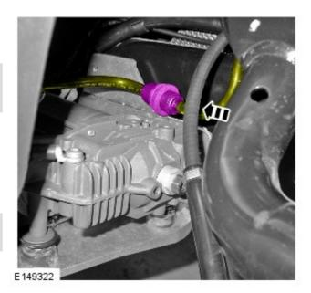
19. CAUTION: Make sure the wiring harness is not trapped between the suspension compressor mounting bracket and the chassis, failure to follow this instruction may cause damage to the vehicle.
