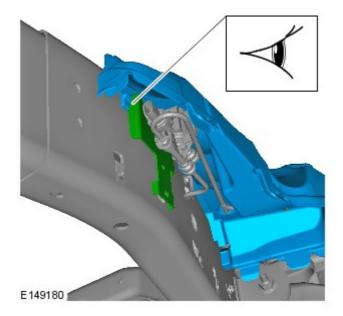
8. CAUTION: Make sure the new pipe is installed securely into the new air suspension compressor connector, failure to follow this instruction may cause damage to the component.
