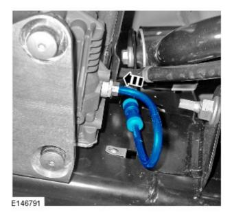
**33.** Connect the new air line link pipe.
