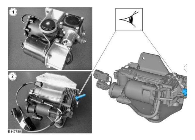
NOTE: Vehicles equipped with Hitachi air suspension compressor.
