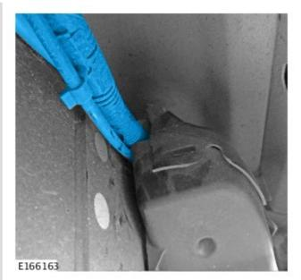
**20.** Connect the air line and the 2 electrical connectors.
